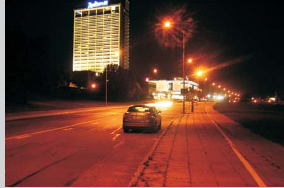
High Pressure Sodium Street Lighting
